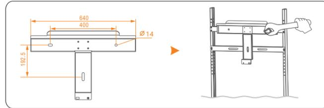
Step 2 Mount the inverter on the rear panel and tighten the inverter with the rear panel by locking screws at the bottom of the inverter.
