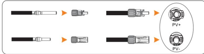
**WARNING** When taking out DC connectors, please ensure that PV Strings are disconnected; otherwise, a fire can occur.
