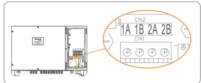
Interface of RS485 communications cable is in the right case of the inverter, shown in above figure.
