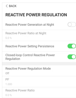
figure 7-16 Reactive Power Regulation
